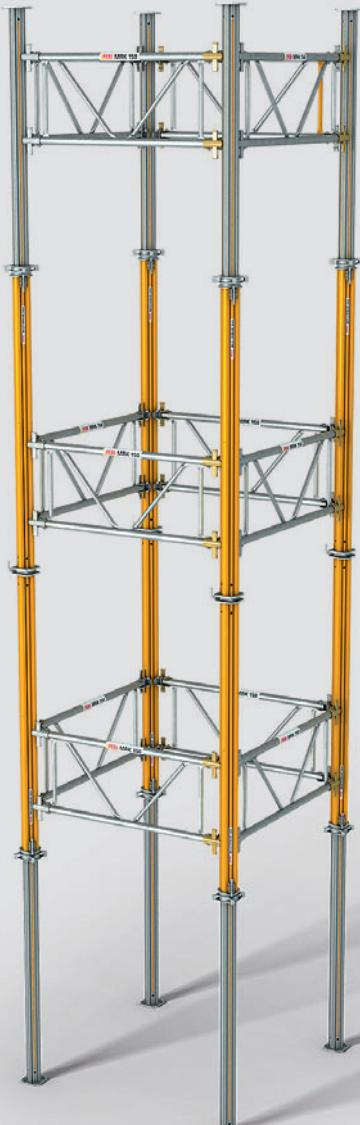
Type-tested assembly as shoring towers with Frames MRK up to heights of max. 14.40 m or 14.90 m with Base MP 50.
