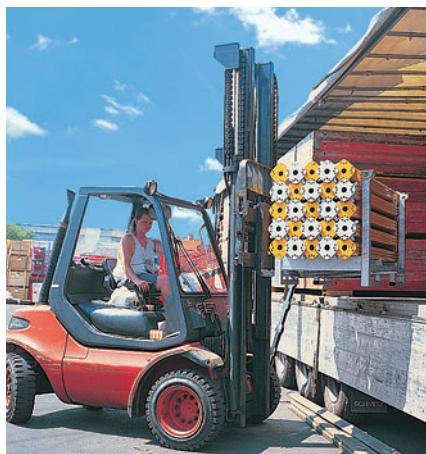
PERI Stacking Pallets are matched to suit truck loading dimensions. They can be lifted using the longitudinal as well as end sides.
