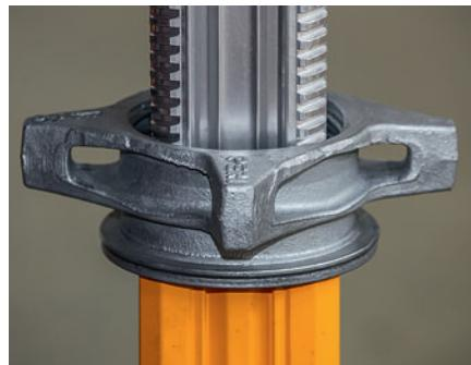
The design of the impact cam on the adjusting nut provides the direction, which is hit using a hammer in order to release a load.
