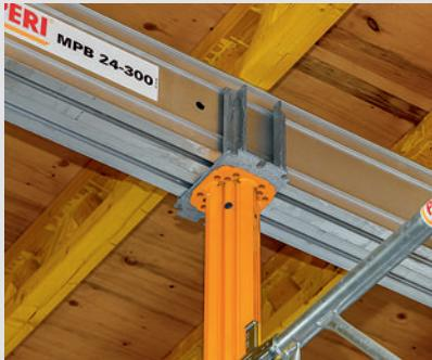
MULTIPROP towers with aluminium MPB Beams as main beams and GT 24 as decking support. Tilting Forkheads provide secure, non-tilting support for the beams.
