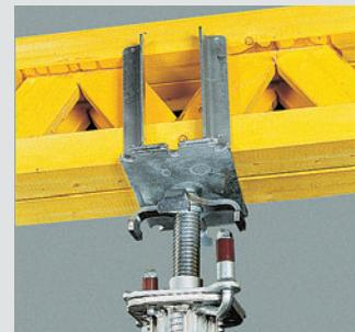
For secure and non-tilt acceptance of 1 or 2 GT 24 or VT 20 Girders. Can be pivoted on all sides by 3°.
