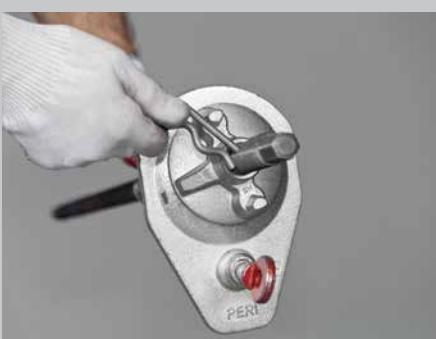
Set out the required wall thickness at the tie by means of a cotter pin, and counter lock with nut. The usual wall thicknesses are indicated through markings on the tie rod.
